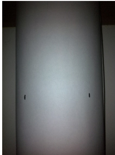
Fig 4: Image, at 1936 x 2592 pixels, of a cylinder of 110 mm diameter as obtained using a mobile phone camera with illumination by the camera flash.
