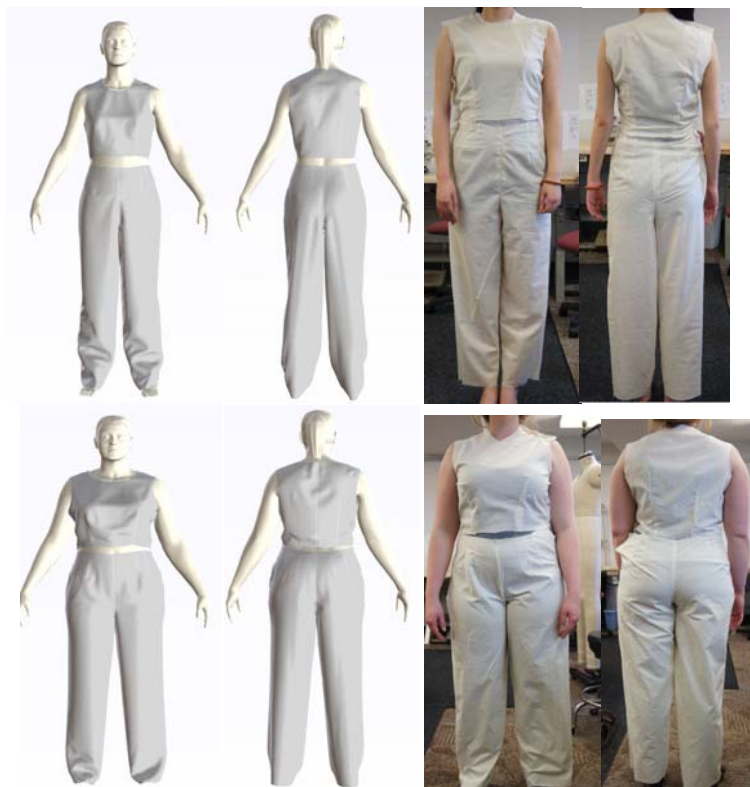
Figure 4. Fit testing on virtual model and live fit model for size 8 (up) size 16 (down).
