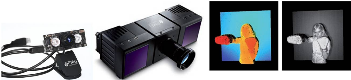
Figure 2: Same technology, two different cameras. PMD Technologies' CamBoard (left) and CamCube (middle). Both cameras provide 204x204 px lateral resolution and an unambiguous measurement range of 7.5m. While the webcam-sized CamBoard was designed as a completely USB-powered solution for the consumer market, the CamCube was designed as a versatile ToF camera with exchangeable receiving optic and illumination unit for manifold applications. To the right a color coded depth 3D visualization and gray value amplitude data is displayed.
